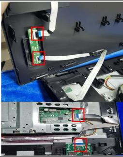
open the cover on the keyboard/ usb board and then pull out the cables
