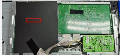
Remove the screws on the mainboard and power board
