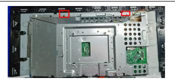
Remove the two screws on the mainframe and then disconnect the FFC cables
