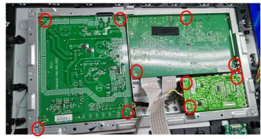
Remove the usb Remove the screw on the usb board board Remove the 3pcs screws on the keyboard Remove the keyboard Remove the screws on the middle frame Remove the middle frame Mainboard and powerboard and coverter board
